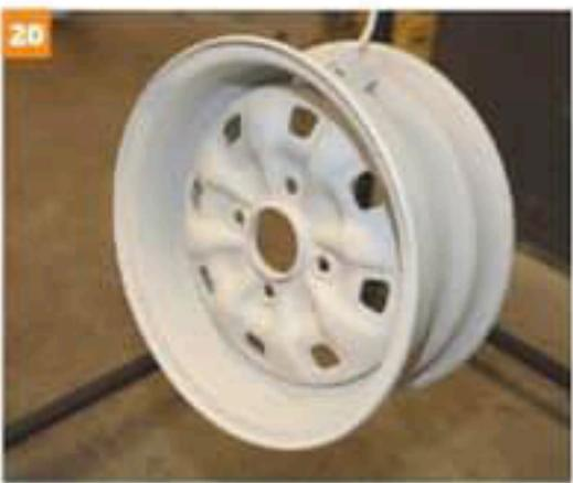
Back in the oven again; to allow all the coats – primer, wet-coat and lacquer to fuse together.
