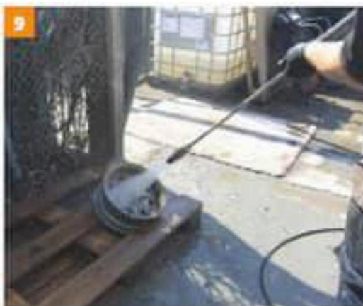
...blasting with a jet wash to clean off any residue and neutralise the chemicals.
