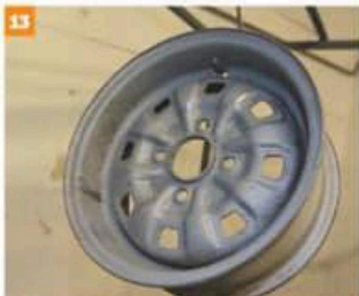
...and wheeled into the oven, to heat the rim to around 200 degrees.
