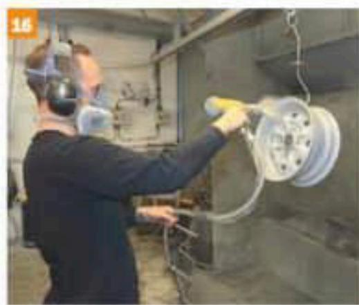
The rim then goes back into the oven, where the powder is melted and fuses together forming a layer for the next stage.
