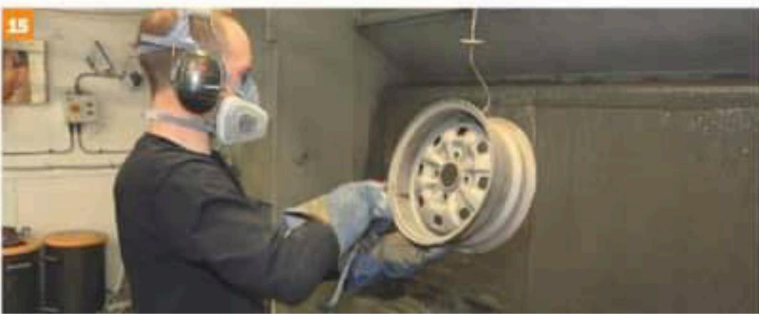
...the first layer of powdercoat primer is added. We're using white here because the colour that will go on top is light. The gun is an electrostatic gun that fires powder at the statically-charged steel rim; making the powder attract and stick to it.
