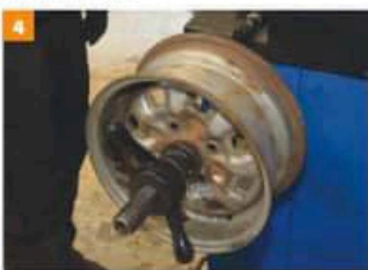
The first job we need to do is spin the wheel up to check its true-ness. Serious wobbles need to be dealt with and Paint It UK have a man that can straighten seriously deformed rims. Luckily ours was acceptable, so we're onto the next stage...
