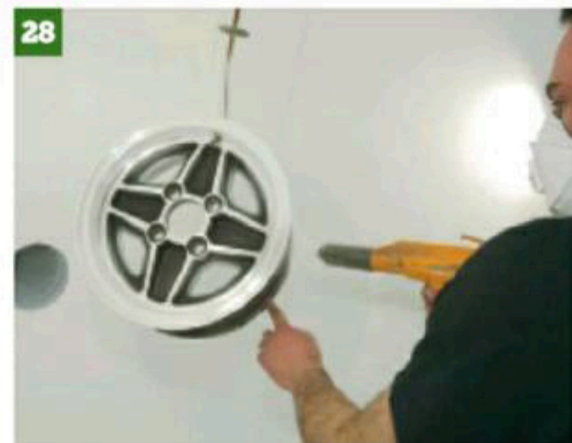
28 When it's coated, the entire wheel goes a milky white – handy because Ash can see exactly where to spray the powder and therefore, not miss any.
