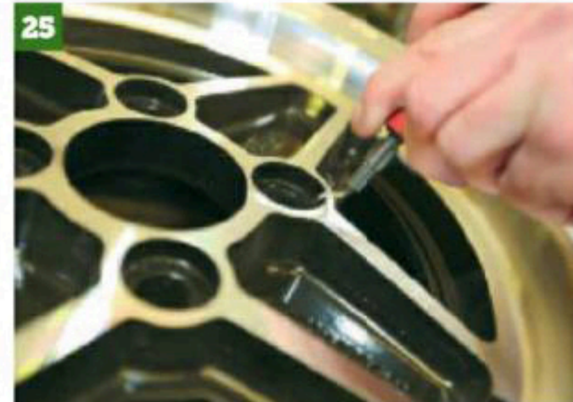
25 Next step is to deburr all the edges, which is done manually with a very sharp deburring tool. This simply rounds the edges over so you can't cut yourself.
