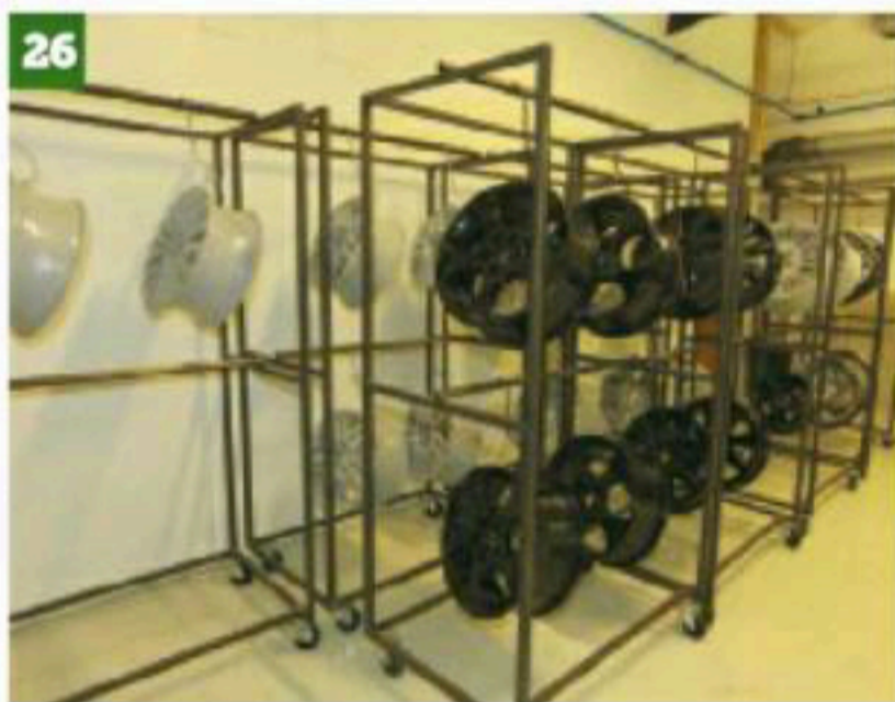
26 The last process begins: lacquering. The wheel is again put into Paint It UK's racks and put back into the oven to heat it to a very high temperature.
