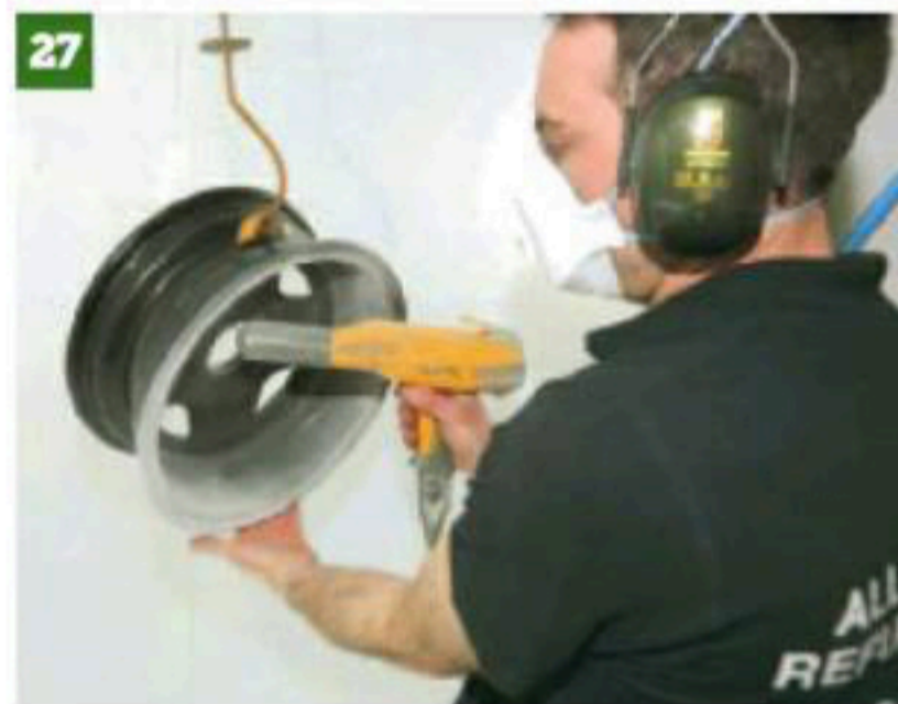
27 Ash uses a completely dedicated, clean booth for this bit, but the lacquering is exactly the same process as the coloured powdercoat.
