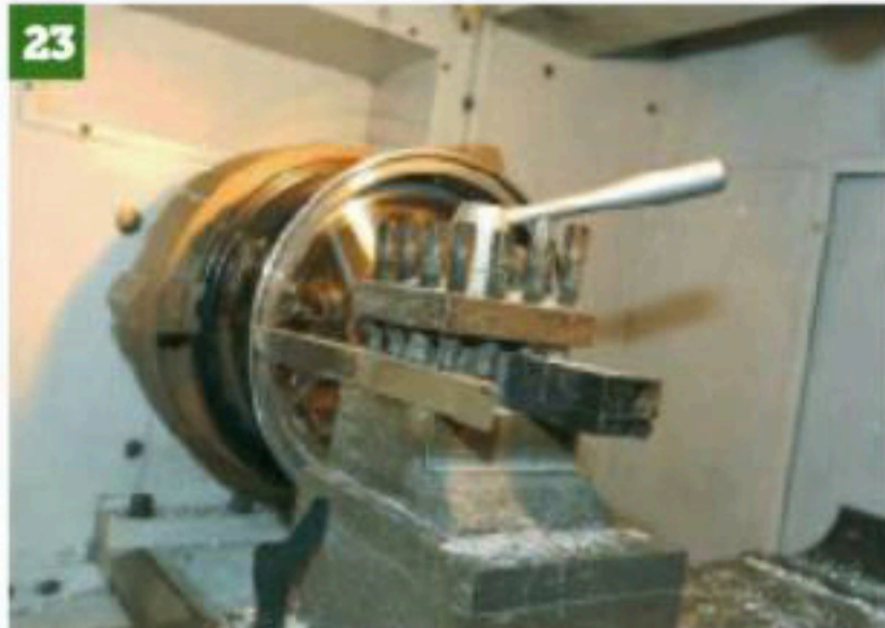
23 It will take several passes to get out all the damage and possible salt staining. It's not an infallible process though – some staining can go way too deep.
